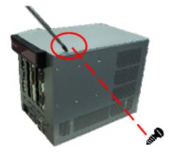
Step 4 Open the top cover and locate the Hard Disk Drive from the side.
